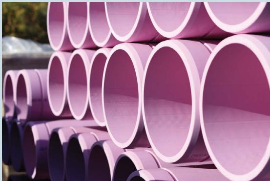
These purple pipes on the Stanford campus carry reclaimed water from sinks and laundry rooms to landscaped areas.
